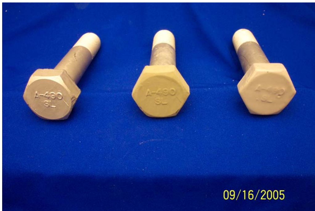
Figure 8: Successive paint steps left to right: unpainted, Carbozinc 11 Primer, and Carboxane 2000
