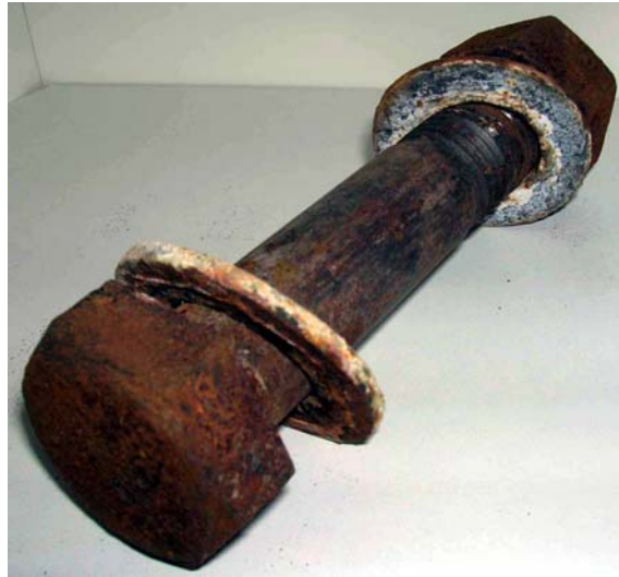
Figure 18: LE spe (Bare + Turn-of-Nut + 120 cycles)
