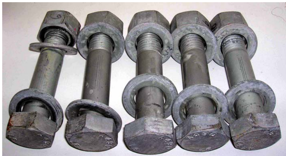
Figure 20: LE spe (DACROMET® + Turn-of-Nut + 120 cycles)
