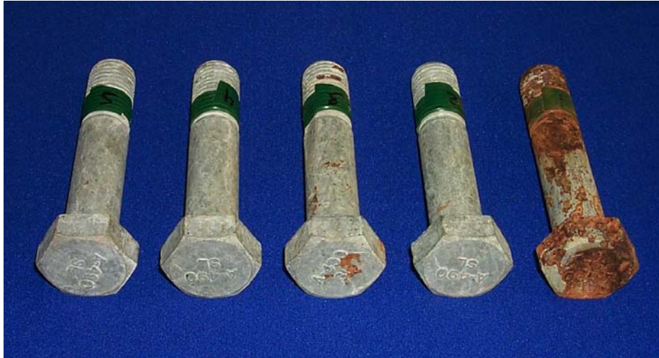
Figure 12: SL std (DACROMET® + 5000 hrs per ASTM B117)
